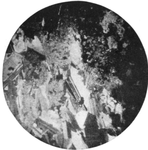
FIG. 3.—Slide showing transition from fresh to altered portion of specimen. \times 25 . Crossed nicols.
